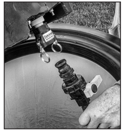
Floatless valve tub disconnected.
